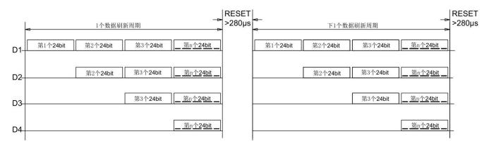
Note: D1 is the data from MCU, and D2, D3, D4 are from Cascade Circuits.
