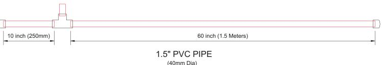
The watering tube is the most important part of this project as it is what will deliver the water to the plants evenly across the entire garden area. The bottom holes are about 1/16 inch (1.5mm) to allow the water to flow out. Above these holes are 3/8 inch (10mm) holes to allow you the option of running string down to the plants.
