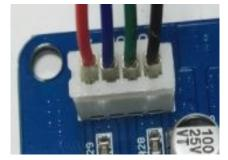
1.use a tweezers pull out the wire from the connector
