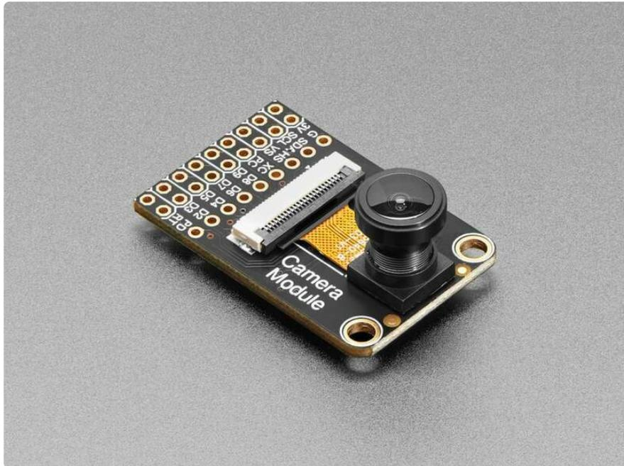
Hobby-level microcontrollers are finally getting powerful enough to start handling camera modules that historically would have required a full computer or FPGA to handle. The RP2040 and ESP32-Sx series of chips, for example, have enough pins to communicate with the 8-bit data output, DMA to quickly grab a frame, and the necessary RAM to buffer a raw snapshot. Now all that is needed is a nice camera module to make interfacing easy!
