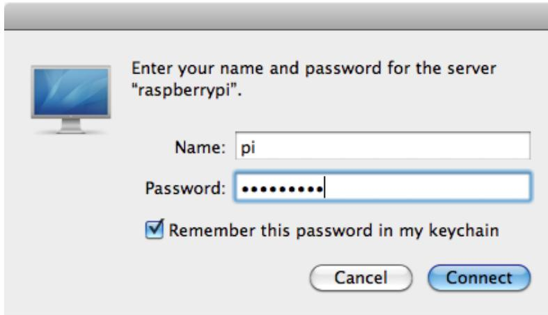
Remember to change the user field to pi and as usual the default password is 'raspberrypi'.
