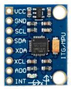
Accelerometers are devices that measure acceleration - the rate of
