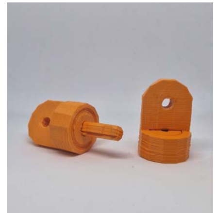
4.3 Connecting pin joint
