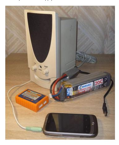
Put the speaker and the battery in a backpack and you are ready to go. Connect via audio cable and play songs form a mobile phone or a mp3 player.
