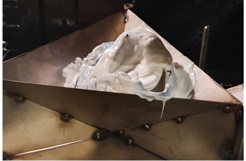
Heat your kitchen oven to approx. 240 °C for PET, PE, PC, ABS, PS and to approx. 210 °C for PLA, PP. Temperatures can be altered but don't exceed 250 °C to avoid dangerous fumes. Open the window and put the negative part of the mould, filled with material, in the oven.
