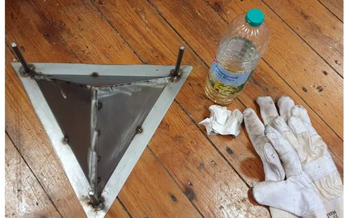
Clean everything: the material you want to melt and the mould. Vegetable oil can be used as a release agent. Grease the inside of both half of the mould with it. Break down the plastic objects in smaller pieces to put them in the mould.
