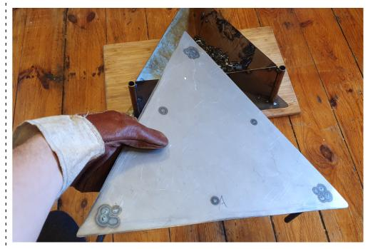
When the material is molten evenly, bring the mould to a well ventilated area and press in the positive part of the mould by hand. Kneeing on it with all your weight helps. After cooling down for 15 minutes release the part from the mould and start again.
