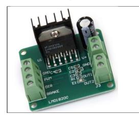
Uses an external LMD18200T module, available on eBay. The LMD18200 supports 3A, the LMD18200T supports 4A.
