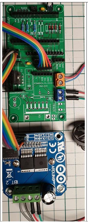
Built up PCB. The orange block is 12v-gnd power in, the blue block is 12v-gnd to the LMD. The grey wires are from the LMD to the track. The R6 wire link is missing in this photo, it should be present.
