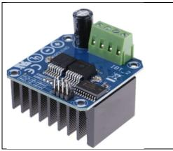
IBT2 board, incorporates two BTS7960B Half-H bridge chips. The board can handle 20Amps+ The System PCB and INA are designed to handle a max 4A. It would be possible to add a shunt resistor in the current measurement circuit to allow the unit to operate at 8A. If you want this much power, then it makes sense to use an IBT2. Otherwise stick with the LMD.
