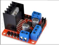
Uses an external L298 module. These are available on Ebay. They also have an on-board 5v regulator which can be used to power the nodeMCU and DSKY option you chose, if any, thus avoiding need for IC1 + C7.
