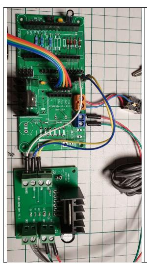
Built up PCB. The orange block is 12v/gnd power in, the blue block is 12v/gnd to the LMD module. The grey wires are from the LMD to the track. The R6 wire link is missing in this photo, it should be installed.
