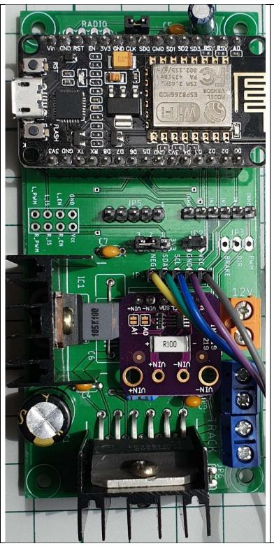
Built up PCB. The orange block is 12v-gnd power in. The lower blue block is power to the track. The upper blue block is unused in this configuration.
