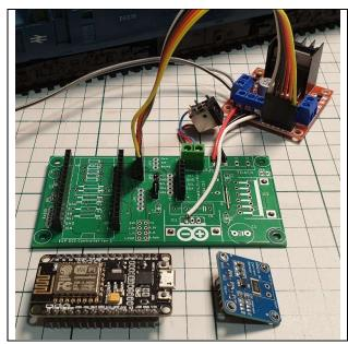
Here's the built circuit board prior to fitting the INA219 and node MCU into their sockets.
