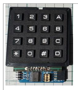
The keypad is a 4x4 telephone matrix. You need to solder on a PCF8574 I2C GPIO expander board (Ebay) to this, the left most INT pin is not required, but there is a convenient hole for it on the keypad PCB. The next 8 pins (P0-P7) pick up the columns and rows of the keypad.
