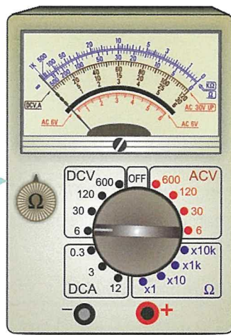
Analogue multimeter set to read voltage
