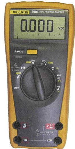
Digital multimeter set to read voltage
