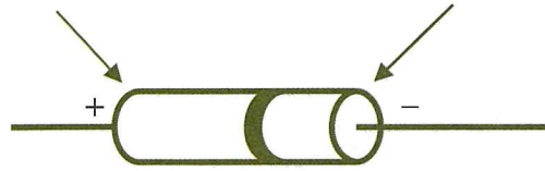
A practical diode – a dark or silver band indicates the negative terminal
