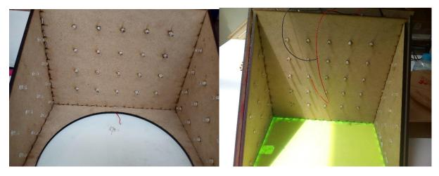
The small triangles are anchors between the inner and outer shells of the box so glue them to make sure that the space between is 5mm.
