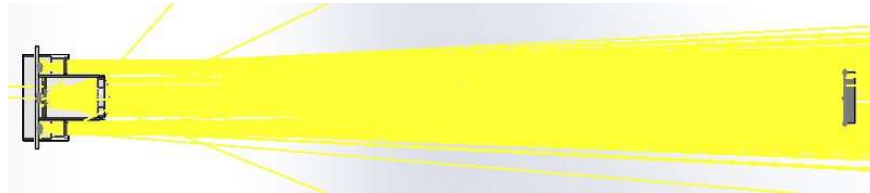
Fig. 1 TF_mini optical simulation of the optical path
