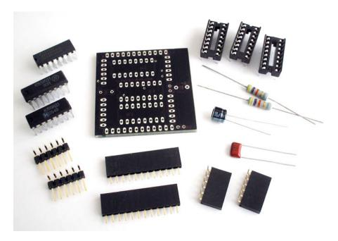
The NIXIE DRIVER board is designed to receive serial input from an external microcontroller (Arduino, etc.) and output decimal information and route power to one pair of nixie tubes. The NIXIE DUO board mounts on top of the NIXIE DRIVER board and supports two IN-12A type nixie tubes via two phenolic sockets. The high voltage requirements of at least eight pairs of IN-12A nixie tubes may be provided by our NIXIE TUBE POWER SUPPLY.
