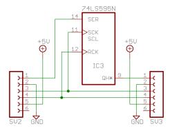
When connecting **NIXIE DUO** boards edge-to-edge, the serial data for controlling the display of digits should enter via pin 1 of SV2. Each board then outputs the serial data stream via pin 1 of SV3.
