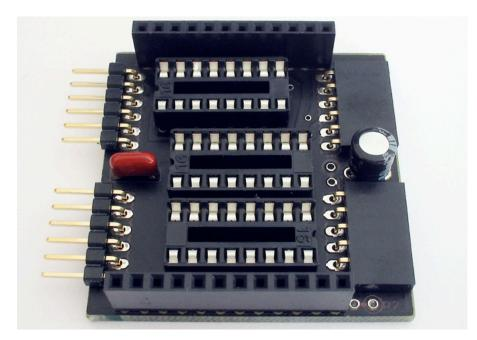
There are two de-coupling capacitors on each NIXIE DRIVER board. Locate C1 on the board, and insert the non-polar metal film capacitor (here pictured red). Solder it in place and trim the leads.
