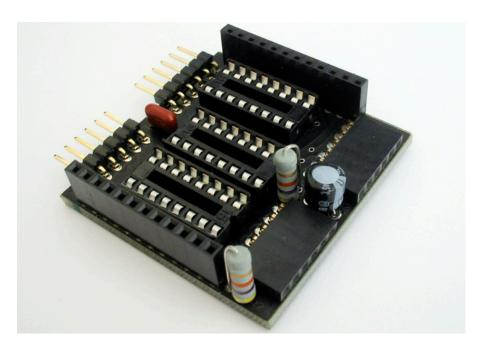
The final two components of the NIXIE DRIVER board are current limiting resistors for the two nixie tubes. R2 and R3 should be prepared for minimum height on the board; doing so will ensure a good seat for the NIXIE DUO board. Turn over one lead of each resistor and insert them vertically into position for soldering. Solder and trim the leads on the reverse side.
