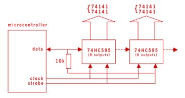
The NIXIE DRIVER permits a microcontroller (Arduino, etc.) to address two nixie tube digits, and via a shift register chain, multiple pairs of nixie tube digits. The 74HC595 shift register is used here to extend the microcontroller output functions.
