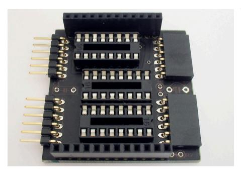
The two straight 12-pin female headers can be added next. You can use the weight of the board to hold these in place while soldering. Similarly, it is a good idea to start with end pins, and check final position, before soldering the remaining pins.
