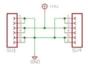
The nixie tube high voltage supply should be presented to pins 3 and 4 of SV1, and will then also be present on pins 3 and 4 of SV4.
