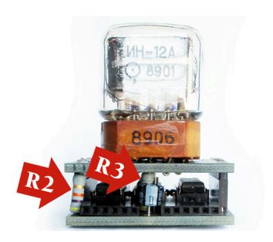
When attaching a NIXIE DUO board above the NIXIE DRIVER board, direct the top of R3, as shown, into the hole in the board above. This prevents accidental contact with the nixie tube pins. Also, slightly bend in R2 to permit the two boards to seat flat.
