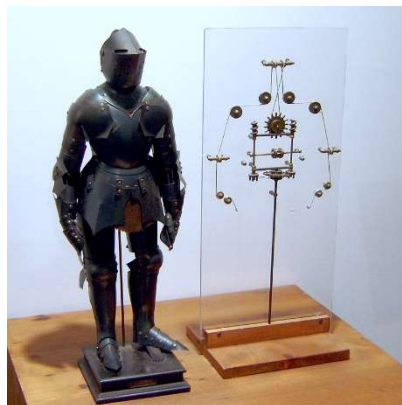
Fig. 2.1 Model of Leonardo's robot with inner workings
