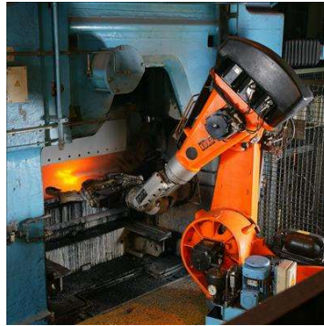
Fig. 2.4 A pick and place robot in a factory
