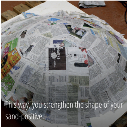
You can cover the newspaper-coating with some extra layers of wrapping film.
