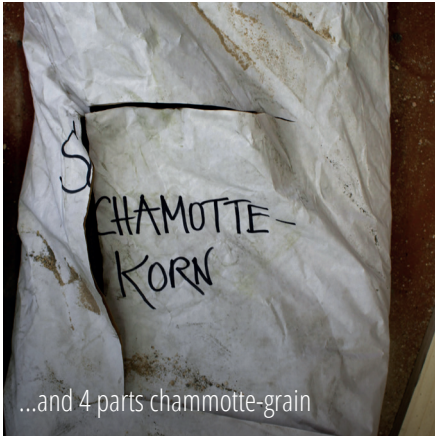
This way, you strengthen the shape of your sand-positive.
