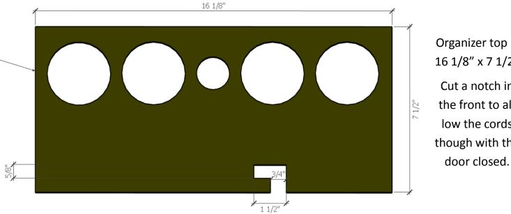
Organizer top is 16 1/8" x 7 1/2" Cut a notch in the front to allow the cords though with the
