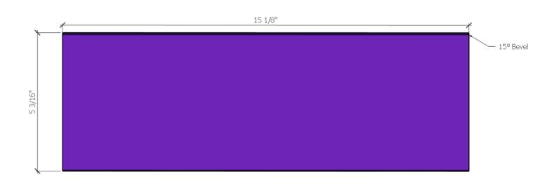
Bottom of the storage unit is 15 1/8"x5 3/16" with a 15° bevel on that will be the front of the bottom piece.
