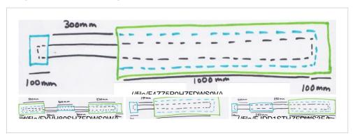
All normal Pompfen use the same construction process described in Step 2. In this step, we've provided schematic diagrams for each Pompfe, with pipe and padding lengths marked clearly. The black is PVC pipe, the blue is the rubber pipe insulation, and the green is the softer foam.
