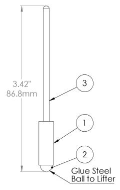
If assembled length is too long or short, scale lifter in the Z axis and reprint.
