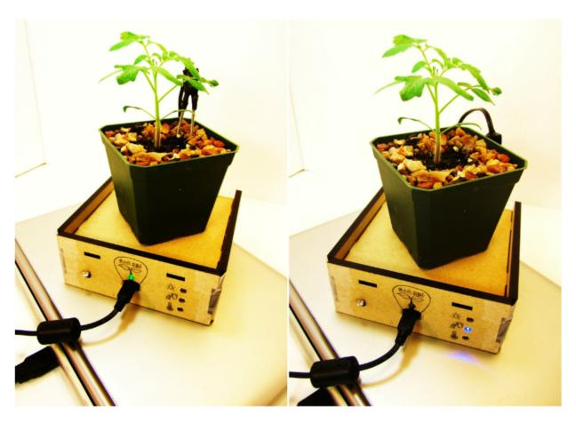
when all conditions are optimal (sun, water, temperature) the plant shelf stays lit green indicating perfect health. if either of the sensors are triggered the corresponding light comes on (sun>yellow, water>blue, temperature>red) and notifies the user to take action.
