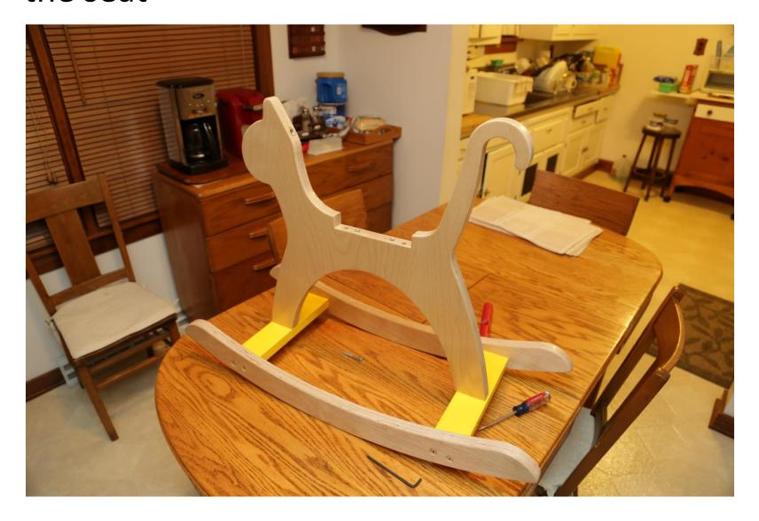
Place the seat as shown. Thread a screw into each hole and tighten.
