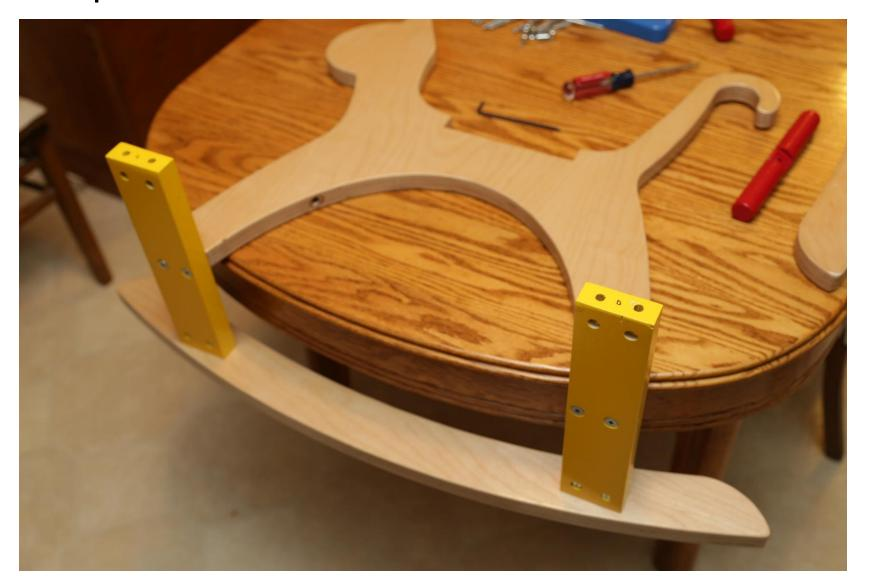
Now, go back and completely tighten all of the screws. Use the long end of the hex key as shown for maximum torque!
