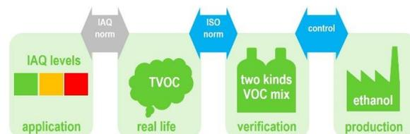
**Figure 5** Production/calibration, verification, and application of SGP30 TVOC sensors. *Blue arrows*: SGP30 sensors are calibrated with ethanol, which serves as a reliable and economical proxy for TVOC.
