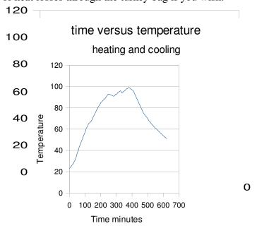
heating I liter water in a 7 I pot the top and sides not heating water
