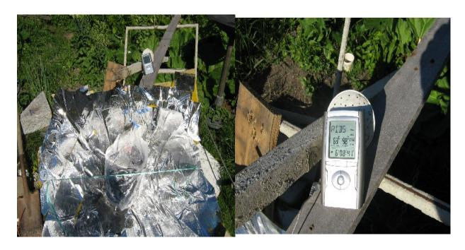
Here is my first test heating 7 liters of water in a 1.25 kg aluminium pot. It was hung at and behind the focal point to try to catch all the sunlight
