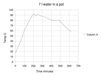
And here is a test I ran on 13<sup>th</sup> september with the same parameters. I let it cool down in the evening after the sun no longer shone on it just to see the cooling curve. This allows an estimate of heat losses through the turkey bag if you wish.
