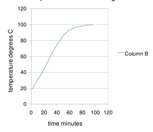
And I also heated soil to steralize it. You should be aware that heat moves through soil slowly so I put the thermometer in the middle at the top. Heat approaches the thermometer slowly! So the curve is not the same as when you heat water!
