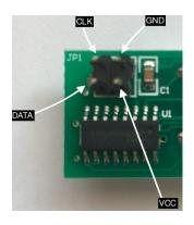
This shows the PIN names on the rear of the display board, as mentioned above.
