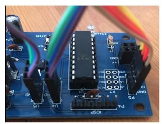
Make sure you connect the leads with the pin names below. The colour of the ribbon cable may vary
