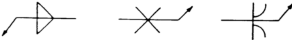
Figure 3-16. Welds on both sides of joint.
