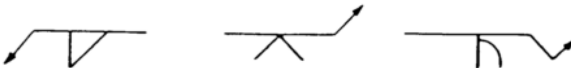
Figure 3-14. Welds on the arrow side of joint.
