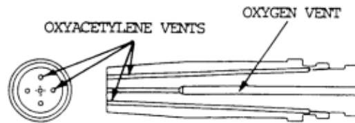
Figure 5-13. Diagram of oxyacetylene cutting tip.
