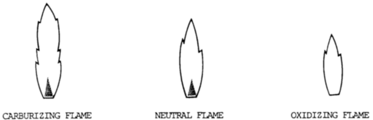
Figure 11-3. What MAPP gas flames should look like.
