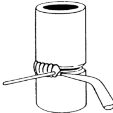
Figure 6-36. Vertical pipe fixed position weld with backhand method.
