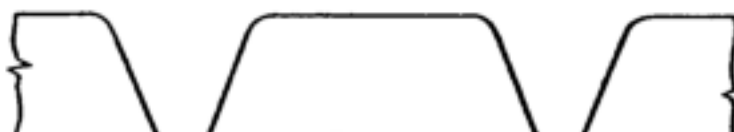
Figure 12-23. Double V plug welding procedure for repairing shell penetration in homogeneous armor plate.
