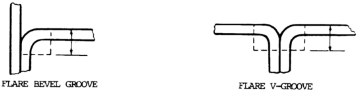
Figure 3-48. Flare groove welds.
