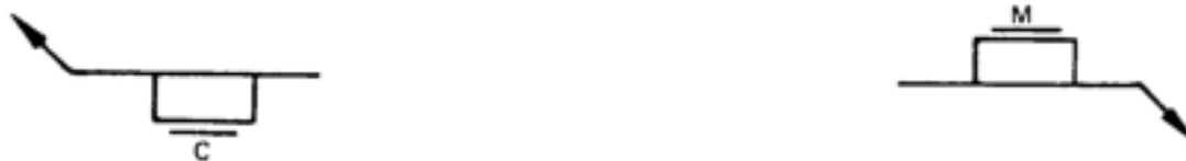
Figure 3-36. Surface contour of plug welds and slot welds with user's standard finish symbol.
