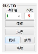
If off-line working of the controller is no longer needed, you can click the button "disable" to turn off the function.
