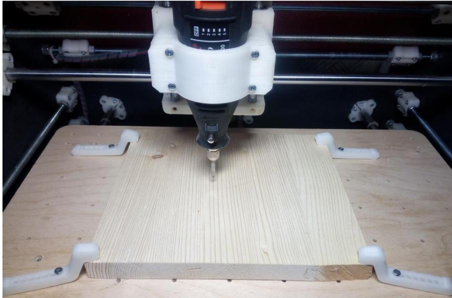
Figure 9 - Workpiece fixing
