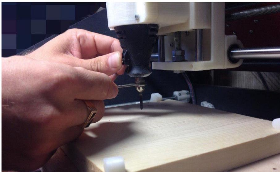
Figure 8 - Installing the cutter.
